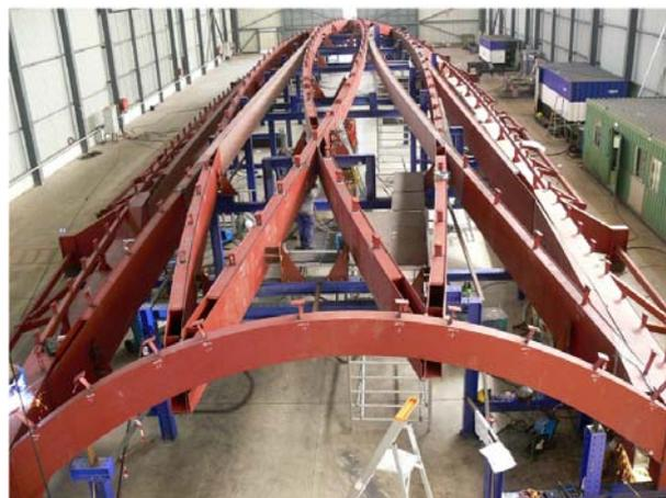
Figure 14: A whole segment of the roof is preassembled in the workshop
