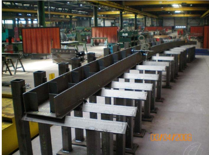
Figure 13: Beam bent in out of plane curvature
